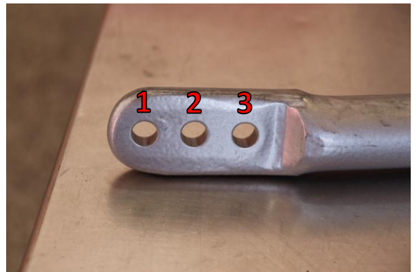
6. Select the sway bar setting by installing the sway bar end link on the end of the sway bar using an 18mm. Position 1 will provide the softest setting. Position 3 will provide the firmest setting.
