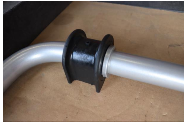
4. Apply the supplied grease to the inside of the new left and right sway bar bushings. Install the bushings on the bar to the inside of the locating tabs.
