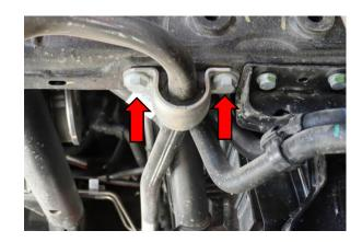
4. Use an 18mm to remove the left and right sway bar brackets. Remove the sway bar from the passenger side of the vehicle. Remove the left sway bar end link from the sway bar.
