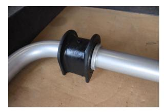
5. Apply supplied grease to the inside of both new sway bar bushings. Install the new sway bar bushings on the Eibach sway bar with the bushings to the outside of the locating tabs. Install the left sway bar end link on the left side of the new sway bar. Tighten to manufacturer specifications.
