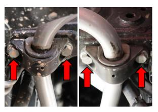
6. Install new Eibach sway bar brackets over both the left and right sway bar bushings. Install the sway bar in the vehicle from the passenger side. Use an 18mm to secure the sway bar brackets to the frame. Tighten to manufacturer specifications.
