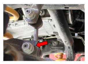
2. Use an 18mm to remove the driver side sway bar end link on the axle side of the link.
