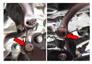
8. Install the axle end of the left sway bar end link using an 18mm. Install the sway bar end of the right sway bar end link using an 18mm. Tighten to manufacturer specifications.
