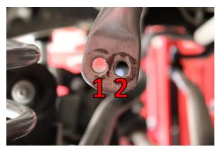
7. Select a sway bar setting during sway bar end link install. Setting 1 (rear hole) will provide the softest setting and setting 2 (front hole) will provide the firmest setting.
