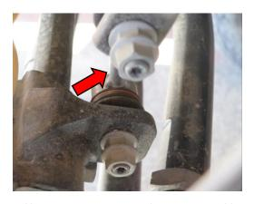
3. Use an 18mm to remove the passenger side sway bar end link on the sway bar side of the end link.
