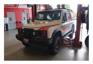
1. Lift and support the vehicle. Remove both front wheels using a 21mm.
